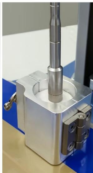
Clamp for stabilizing the sample
