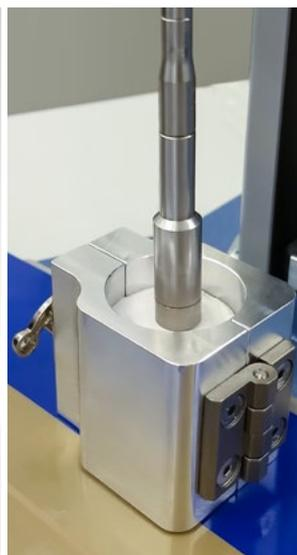
Clamp for stabilizing the sample
