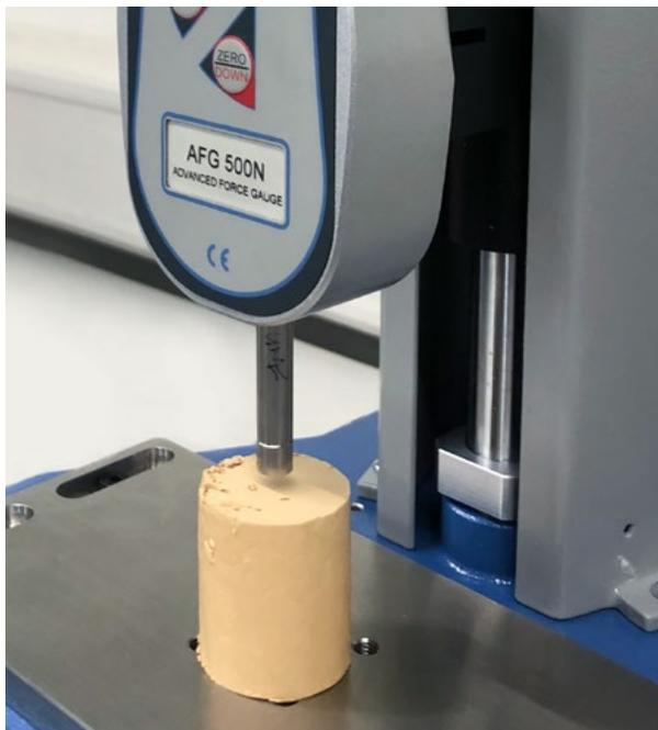
Measuring the deformation pressure
